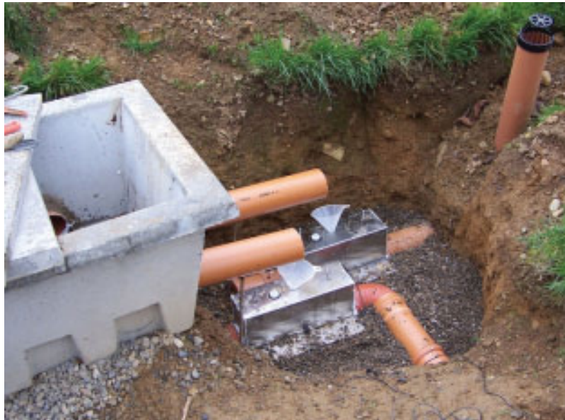
Figure 2.5. Tipping bucket flow gauge instrumentation in place on Site B.
