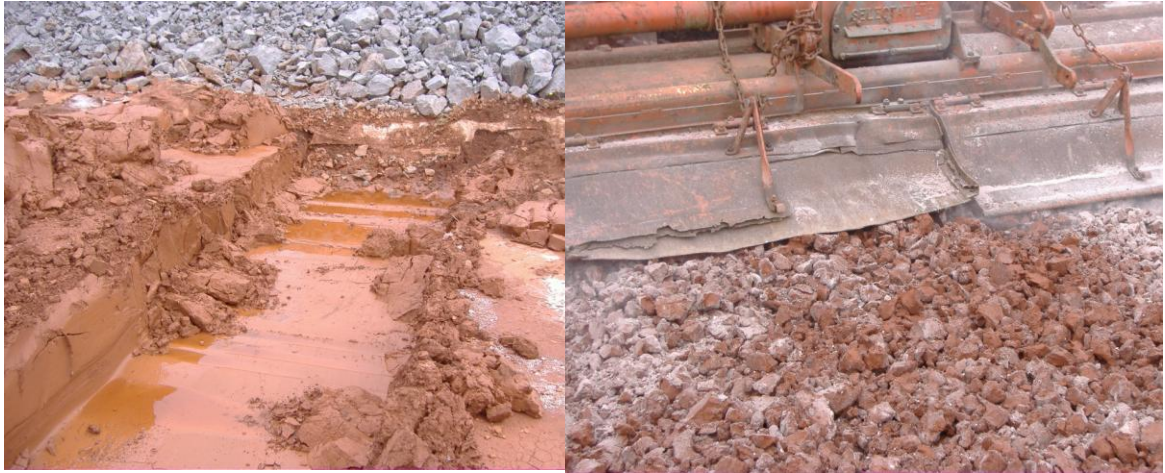
Figure 2. Improving the physical and chemical properties of bauxite residue prior to revegetation
