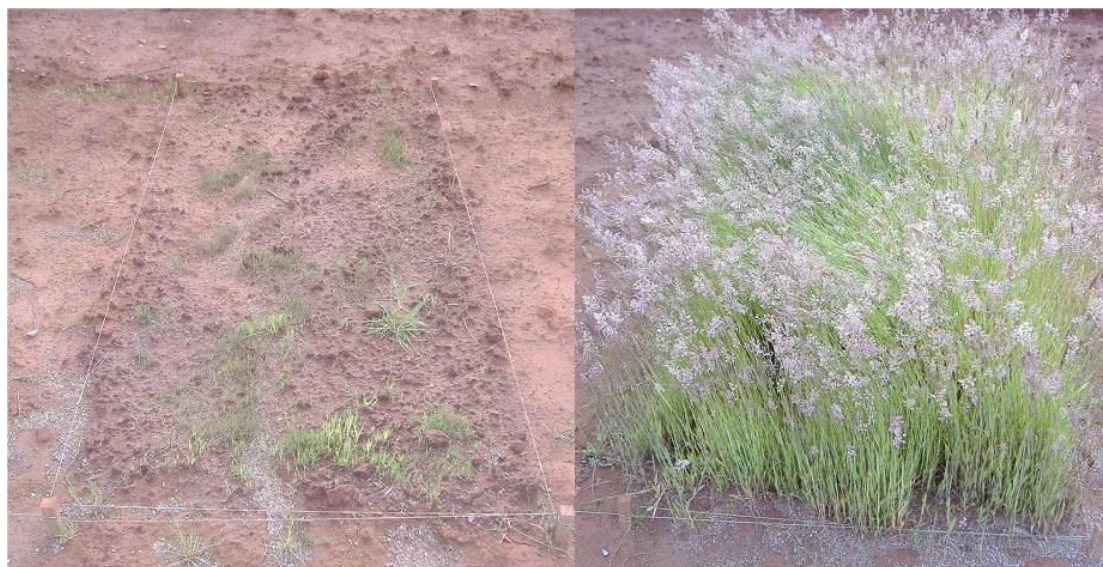
Figure 8. Vegetation grown in amended bauxite residue with organic amendment (right) and without (left)
