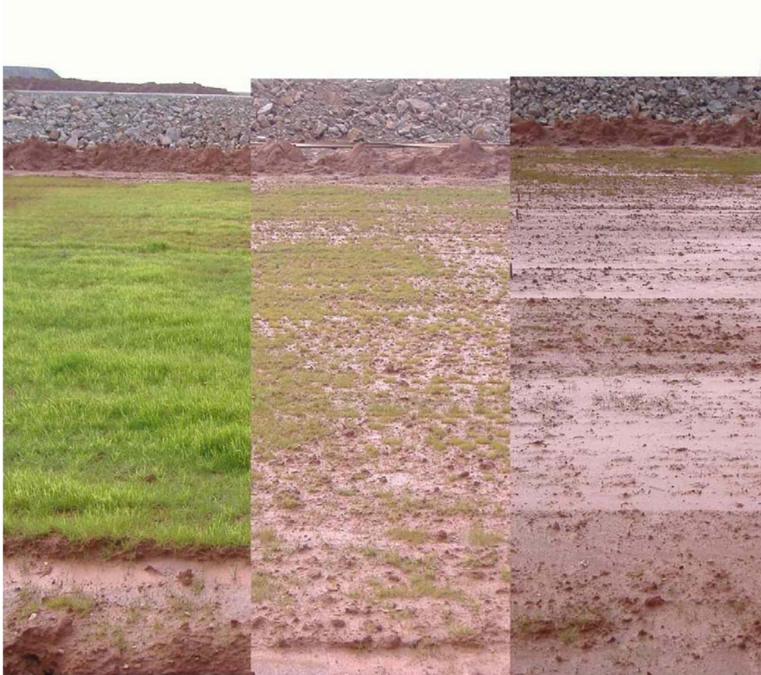
Figure 10b. Different areas of residue from large scale amendment where sufficient amendments were not applied
