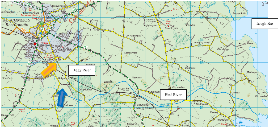
Drawing 3:- Overview of piped treated effluent discharge point to confluence of River Jiggy and Hind. The Hind flows to into Lough Ree. Orange arrow shows WWTP. Blue arrow shows the 1.2km piped discharge location of treated effluent at the confluence of the River Jiggy and Hind from the WWTP.
