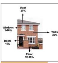
Fig. 4 Heat losses from a house
