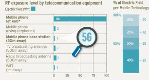
\* Estimate for mobile phone (at ear) based on typical SAR level (1 W/kg), which may be reached in low-coverage situations.
