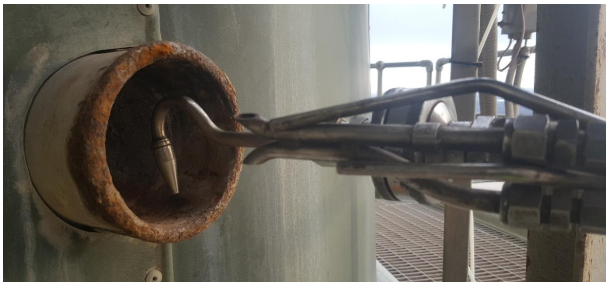
Figure 4: Sampling ports shall allow the insertion and regress of the necessary sampling equipment for isokinetic monitoring preventing any contact that may lead to cross contamination. The picture shows the front end of the sampling probe (sampling nozzle, pitot tube, filter holder).
