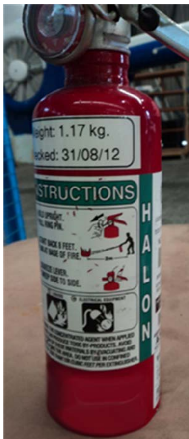
Figure 1: Halon Fire Extinguisher
