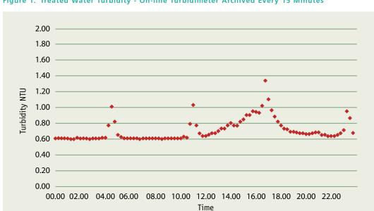
Figure 1. Treated Water Turbidity - On-line Turbidimeter Archived Every 15 Minutes
