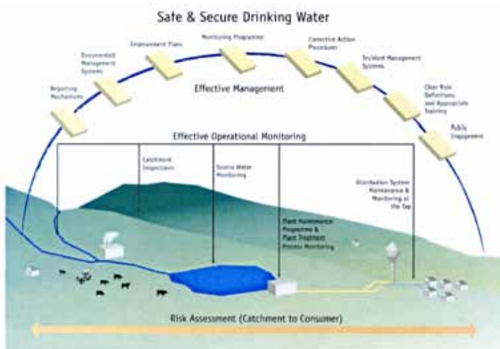
Figure 1: The essential components of a DWSP
