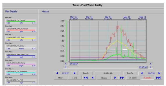
Figure 1: SCADA graph showing the impact on final treated water aluminium levels (red line) and turbidity levels (green line) following the failure of the poly dosing pump.
