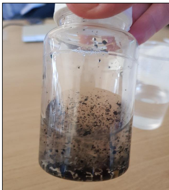
Photo 2: Sample of black particles which caused blockage of alum dosing line, which are thought to originate from the disintegrating lining of the alum storage tanks
