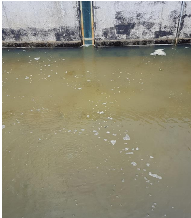
Photo 2 Boiling evident during backwash in a number of locations at Filter 2
