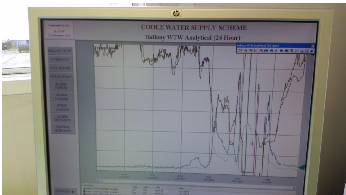
Photo 2: SCADA screenshot showing raw and final water turbidity and UVI trends during a period of raw water quality deterioration (14/11/2014)
