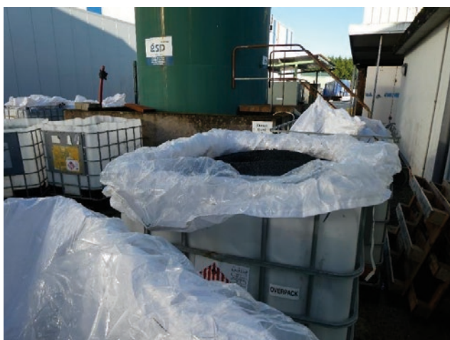
Figure 1 Material stored uncovered outdoors
