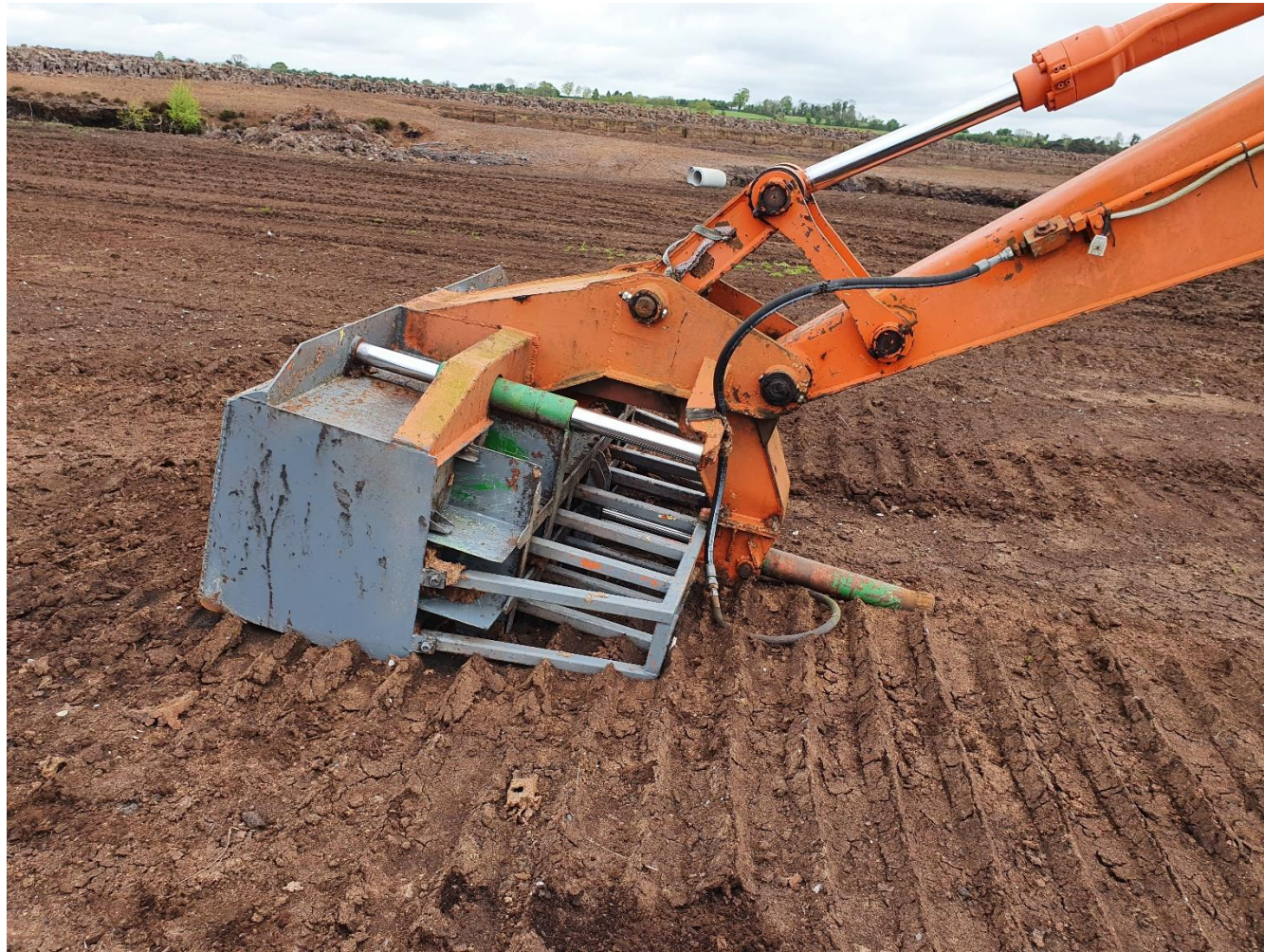
Photo 2: Attachment for excavating sod peat noted.
