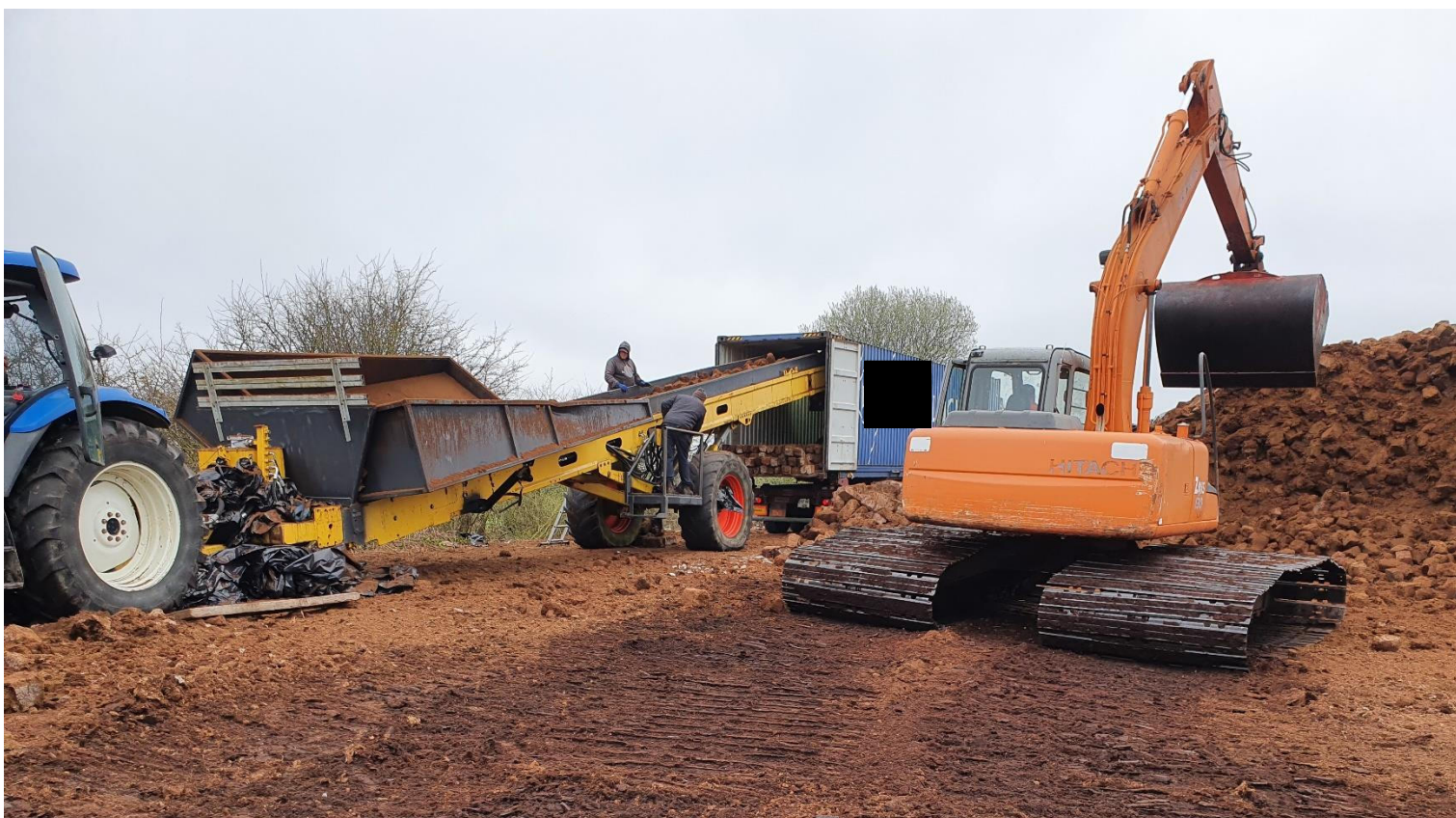
Photo 1: Loading of sod peat on to lorries for export off-site.
