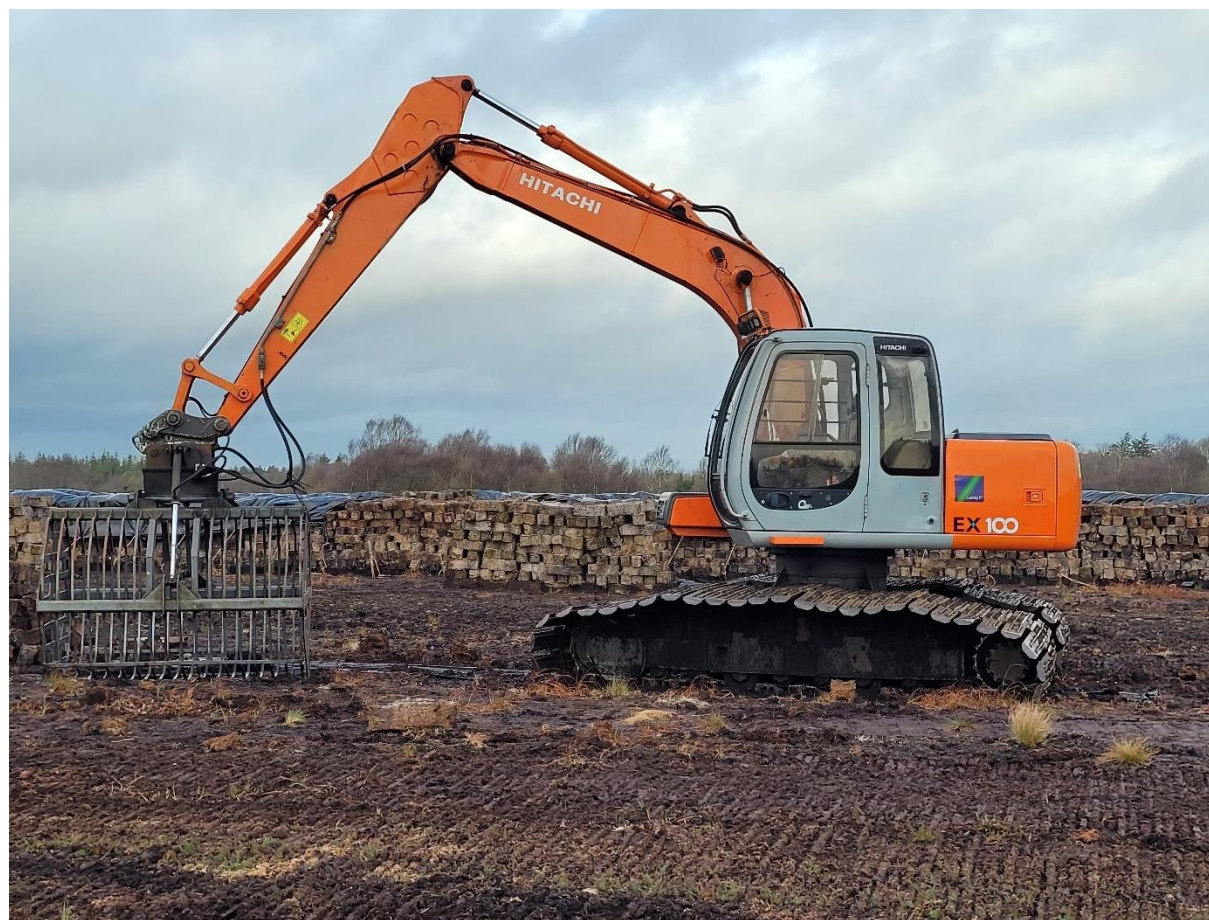
Photo 2: Excavator noted on the peatland with sod peat collector attached.
