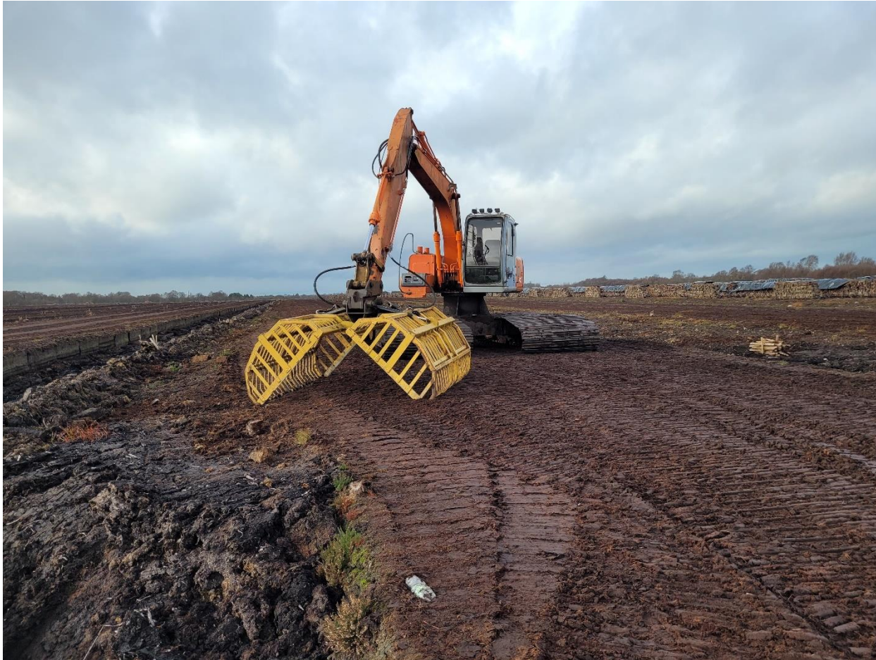
Photo 1: Excavator noted on the peatland with sod peat collector attached.
