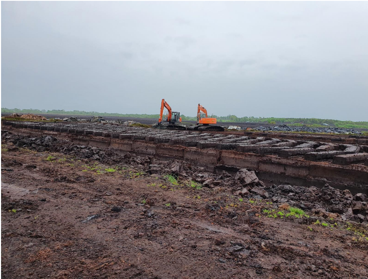
Photo 1: Two excavators extracting sod peat at Area 4.
