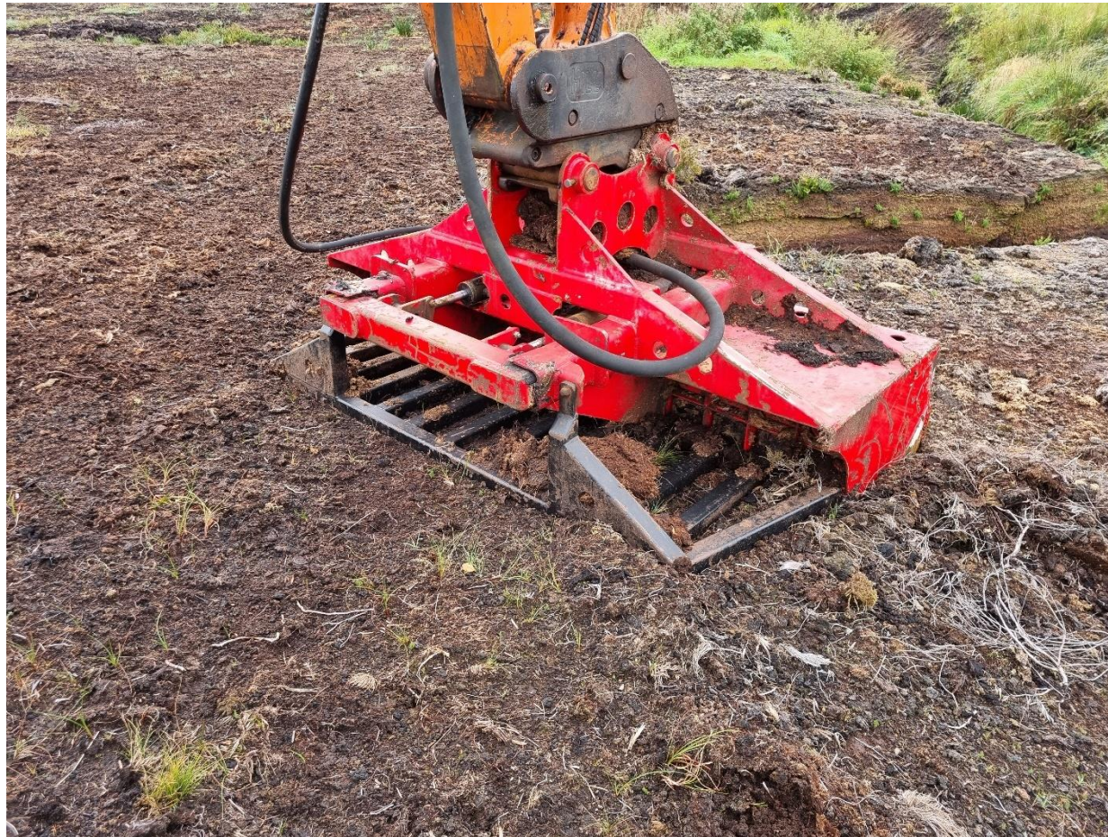
Photo 6: Attachment for excavation of large sod peat noted.
