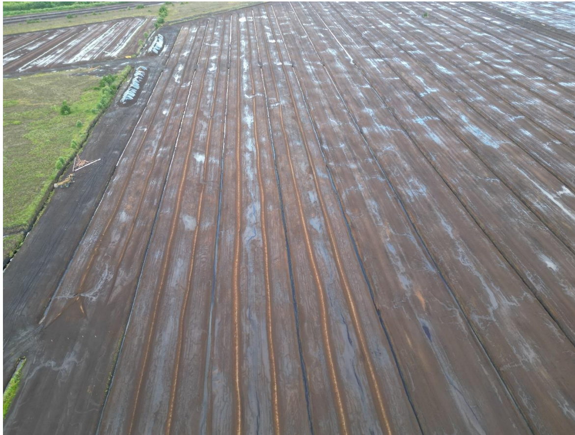
Photo 1: Recent milled peat extraction and harvesting noted on the Southern section of the peatland – Note ridges of milled peat in some rows.
