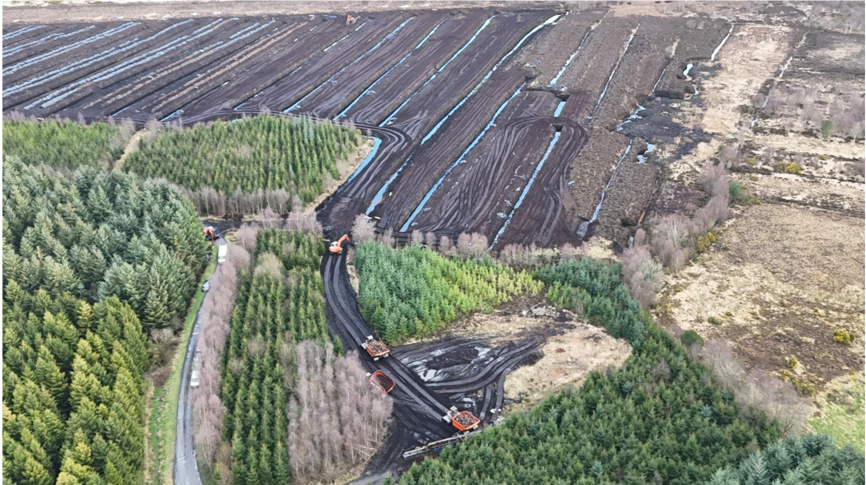
Photo 7: Photo showing large sod peat which was collected from Eastern Section of the peatland being transported to the loading area.
