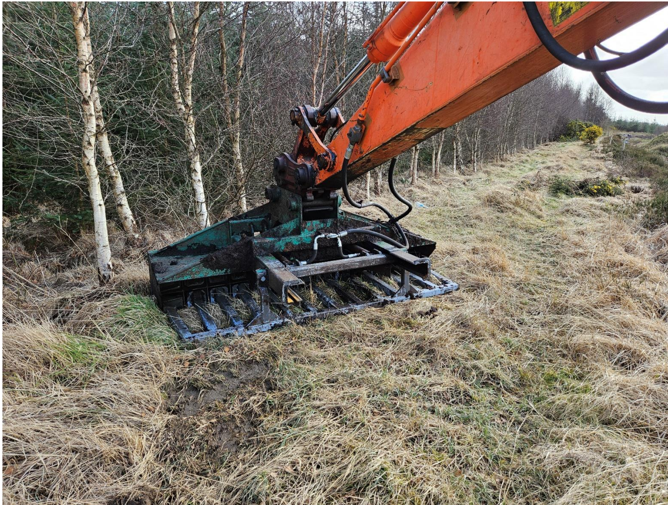
Photo 3 : Excavator with attachment for large sod peat extraction noted at the Western Section of the peatland.
