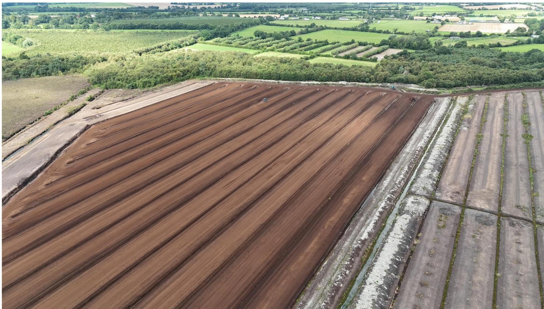
Photo 4: Harrowing of milled peat on the southern/lower section of the peatland.
