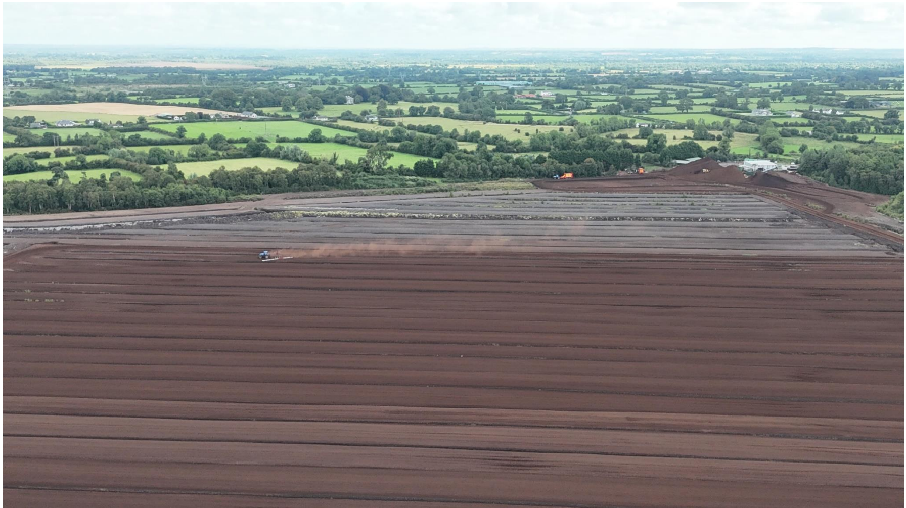
Photo 2: Ridging of milled peat on the central/northern section of the peatland.
