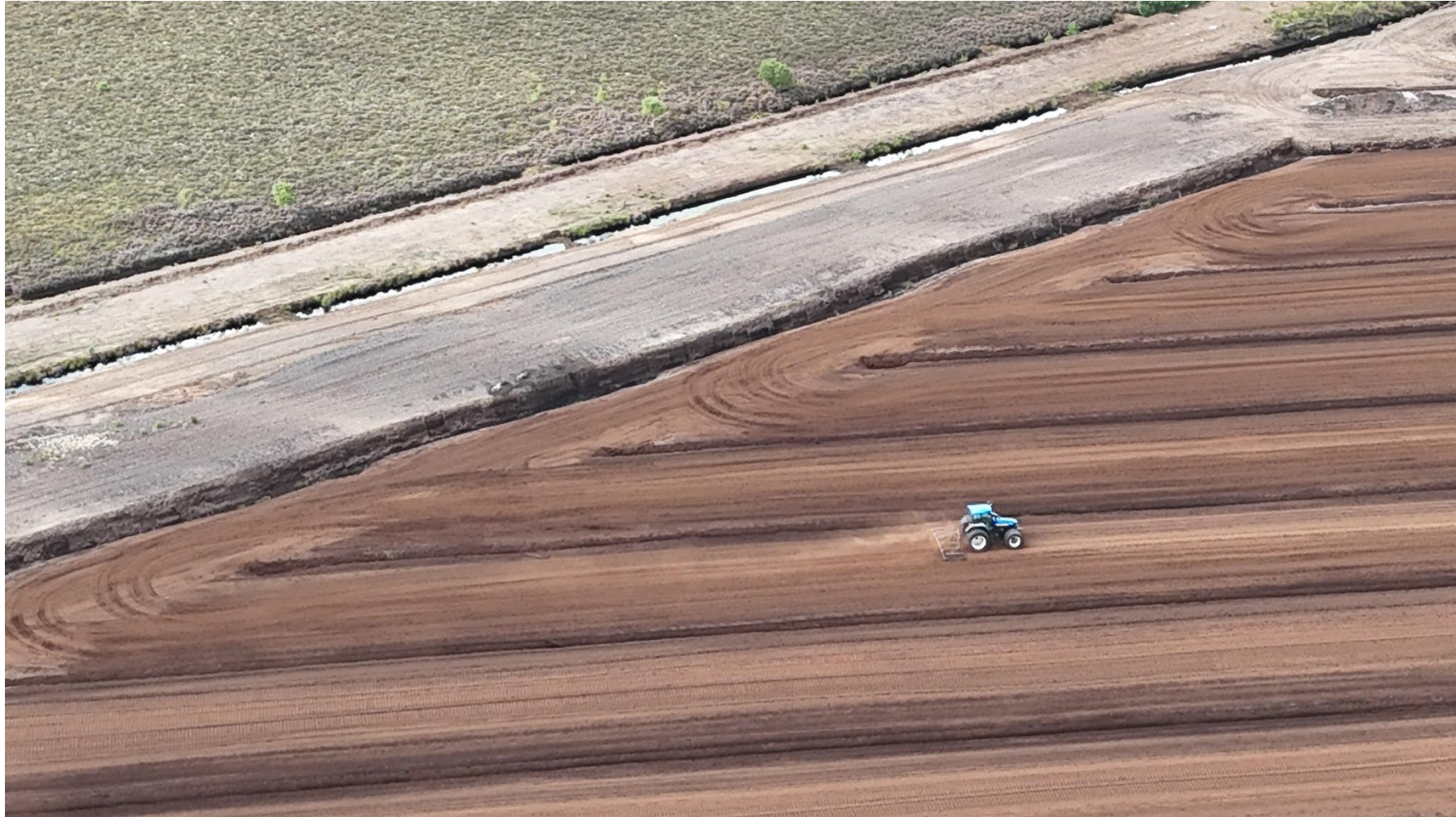
Photo 5: Harrowing of milled peat on the southern/lower section of the peatland.
