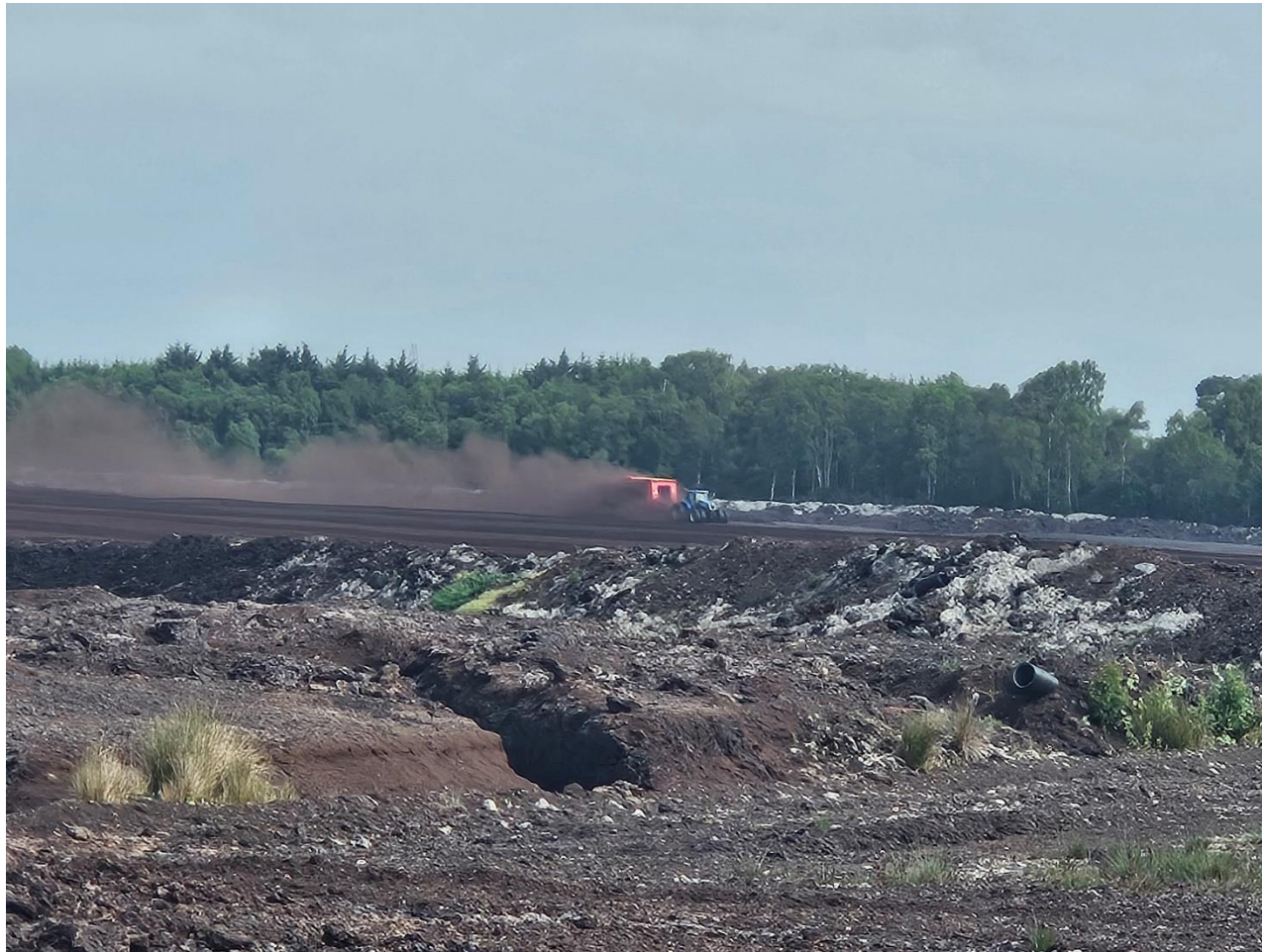
Photo 1: Photo showing the collection of milled peat from the peatland, note significant dust emissions arising.
