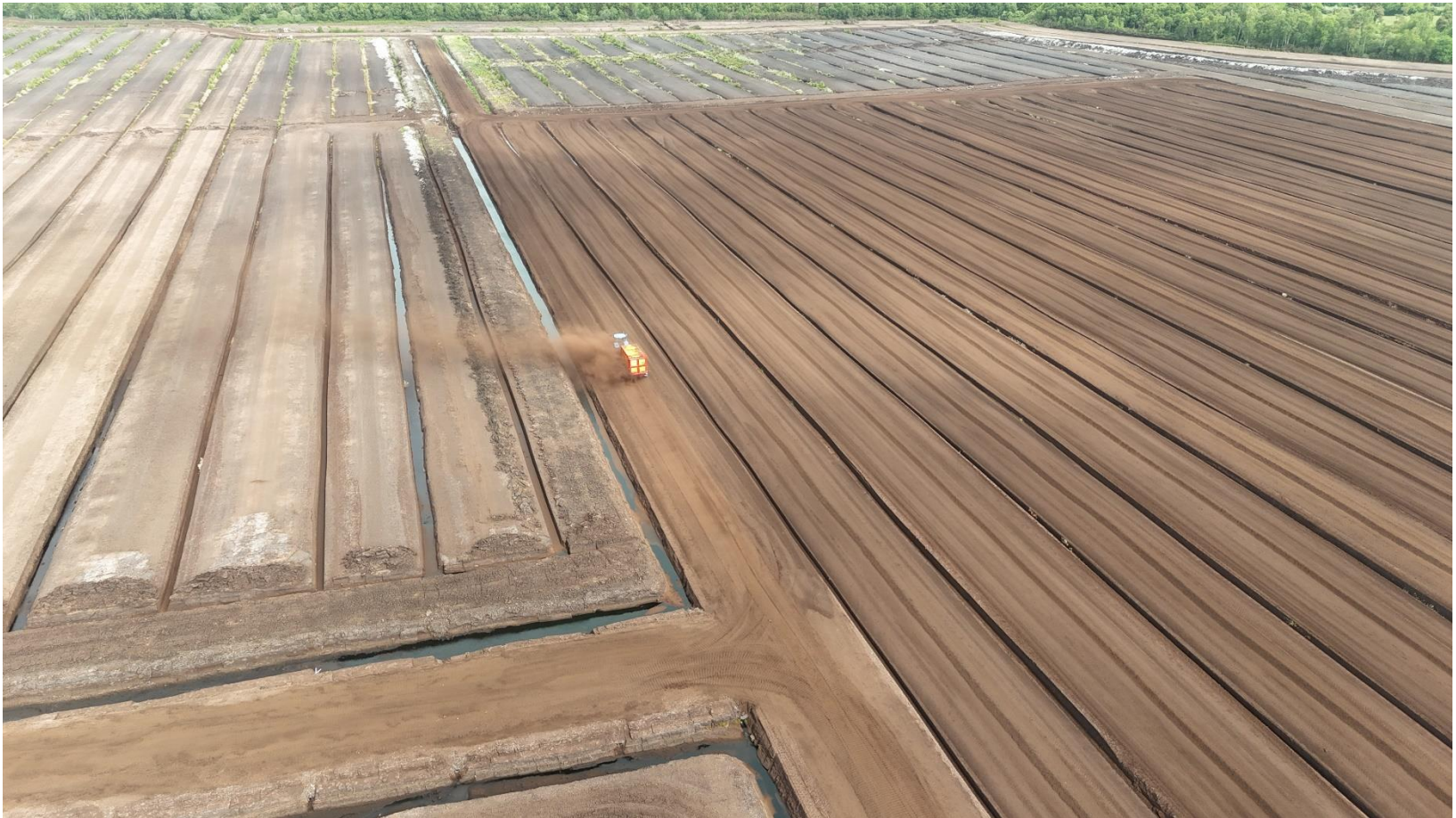
Photo 6: Aerial view of milled peat being collected from the central section of the peatland, note significant dust emissions arising.
