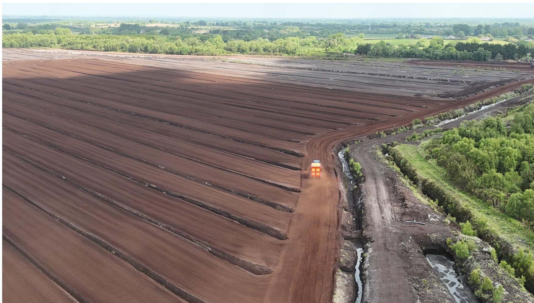
Photo 1: Photo showing the collection of milled peat from the peatland, note significant dust emissions arising.
