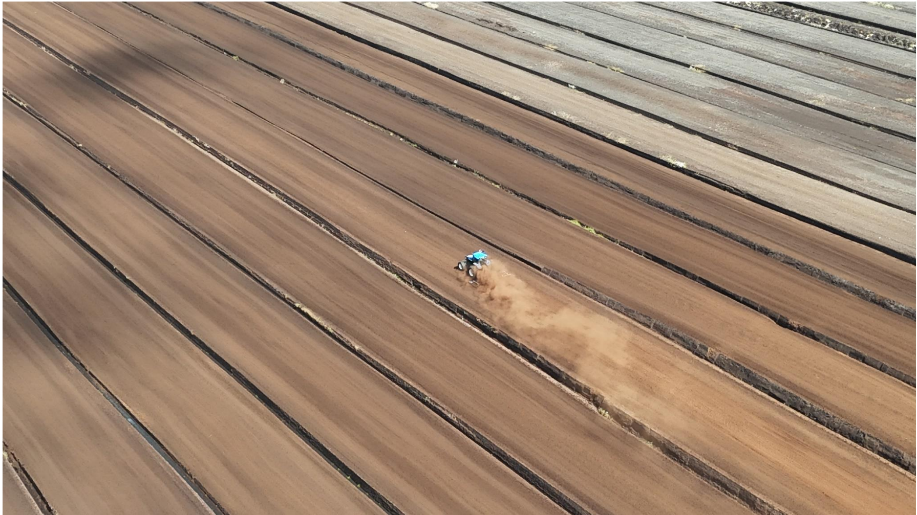
Photo 2: Significant dust emissions noted to be arising from the harrowing of milled peat.
