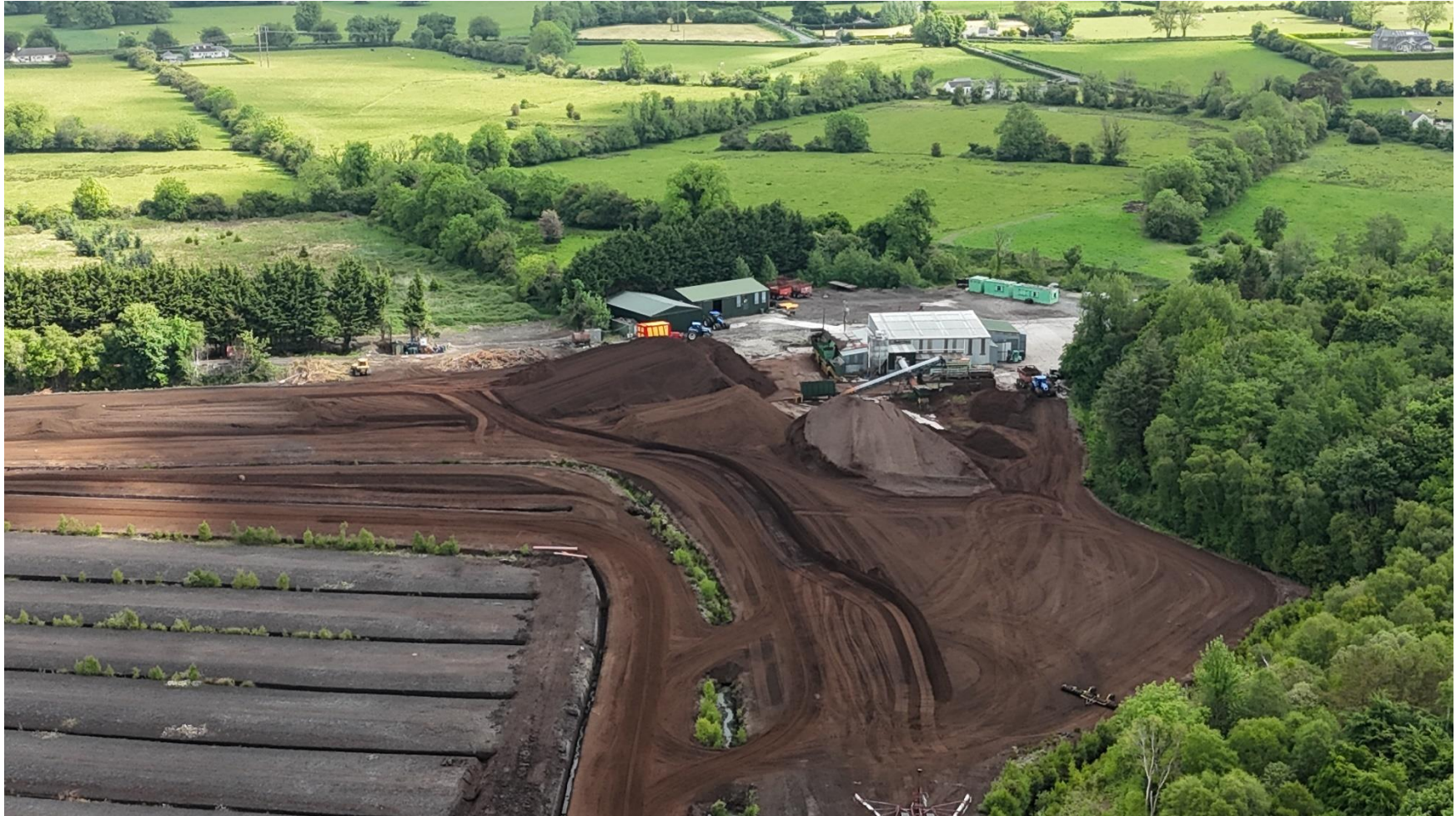
Photo 3: Aerial view of the bagging/processing plant and the stockpiles of milled peat.
