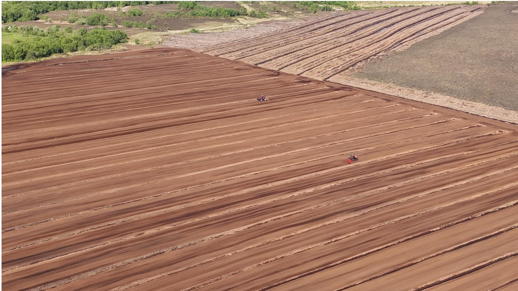
Photo 1– Milled peat extraction noted to be taking place on the western section of the peatland during the visit.
