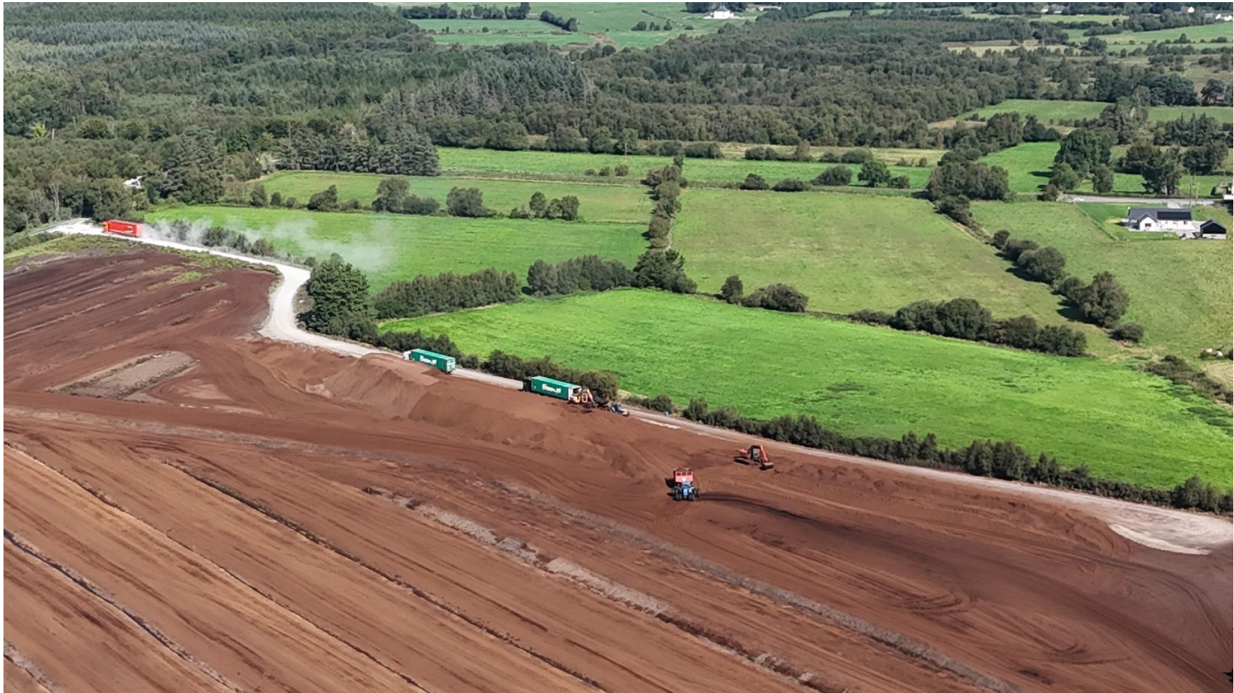
Photo 3: Aerial overview of loading area, note filling of articulated vehicle(s) adjacent to the stockpile of milled peat at the northern end of the peatland. Also note significant dust emissions from articulated vehicle departing the peatland.
