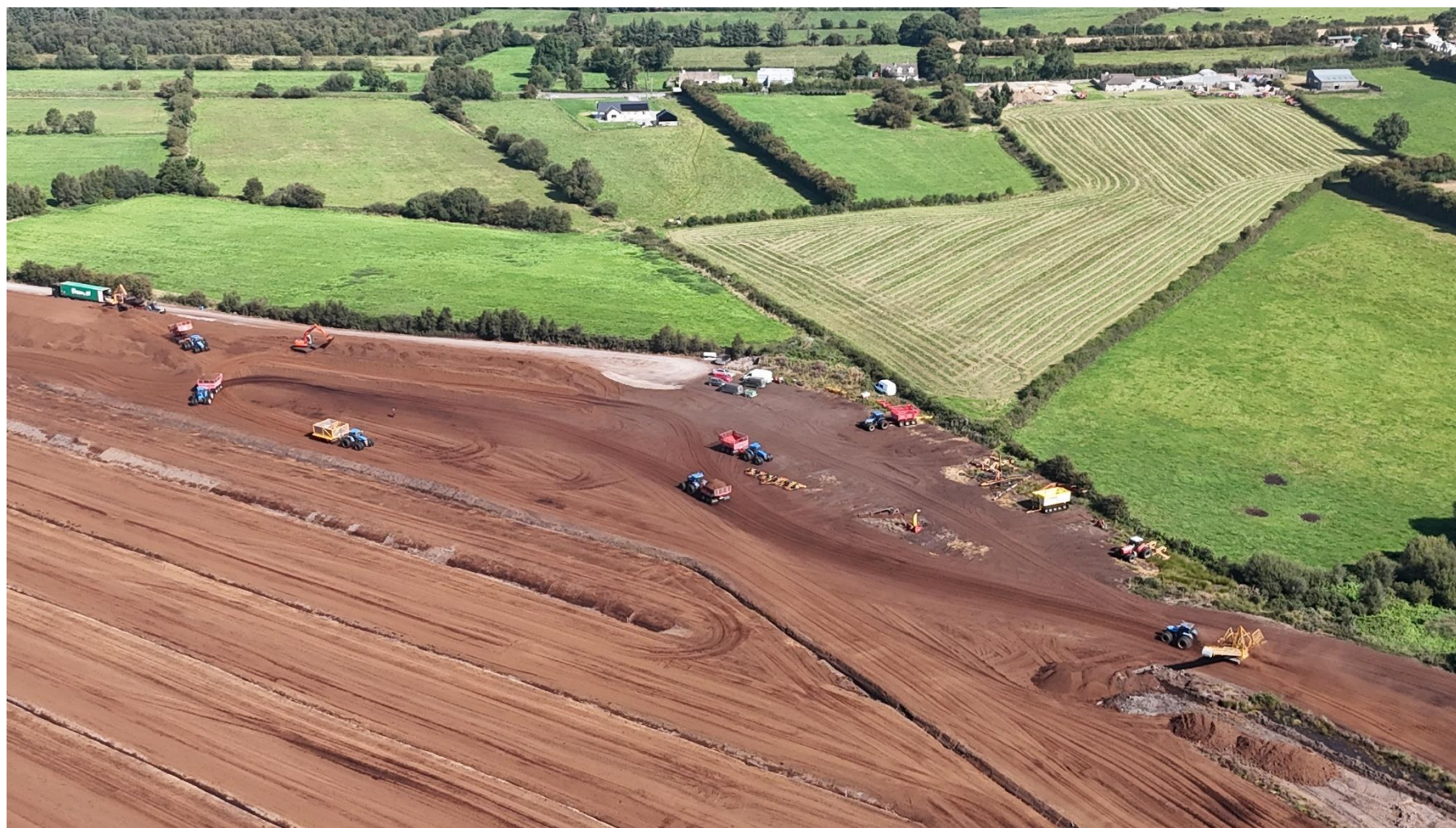
Photo 4: Aerial footage showing the transport of collected milled peat to the stockpile at northern part of the peatland.
