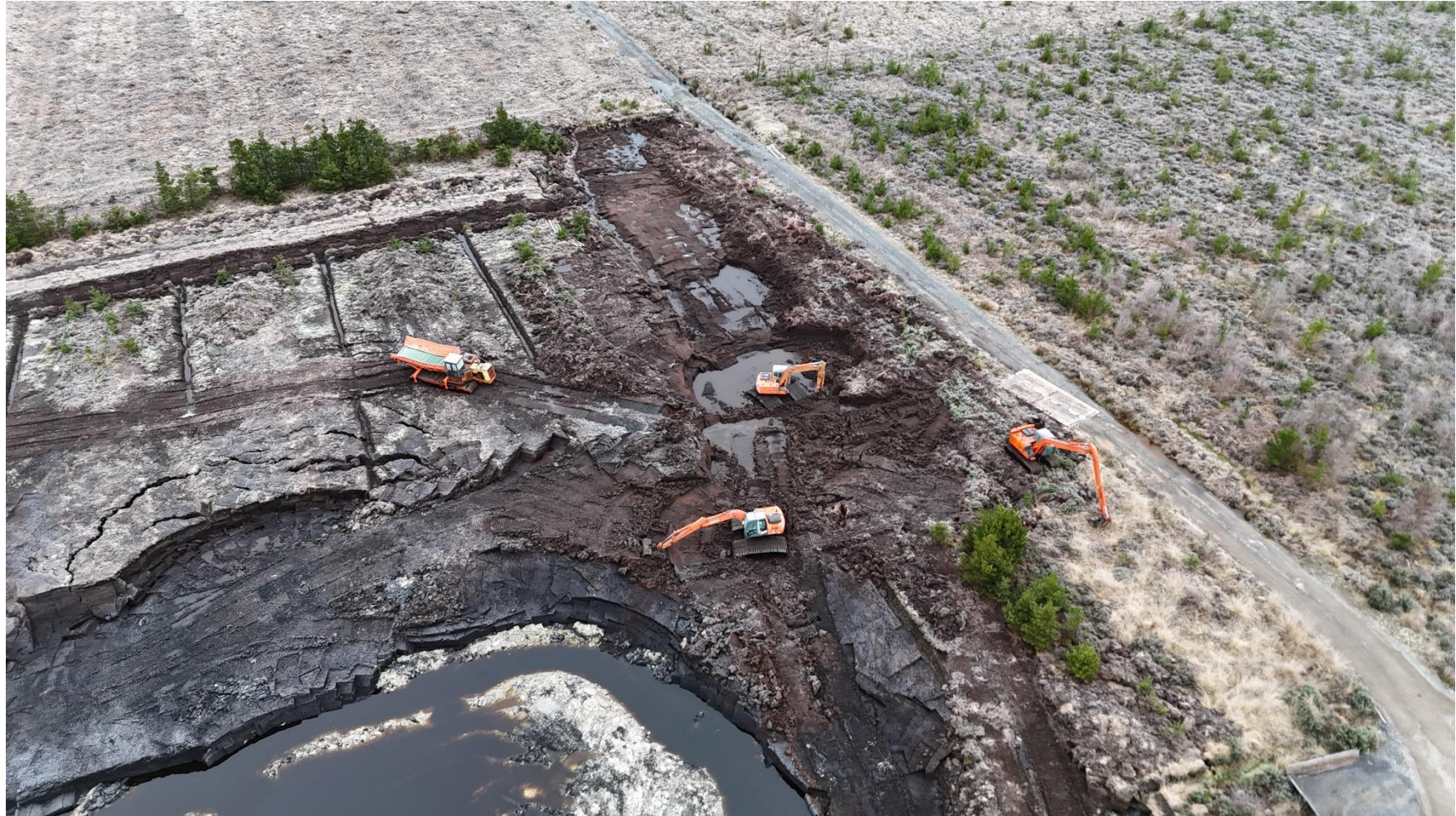
Photo 3: Photo showing peat excavation and transport machinery, area where peat had recently being excavated and road network.
