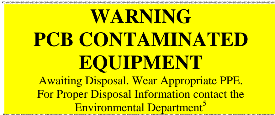
Figure 4: Label for confirmed PCB-contaminated equipment
