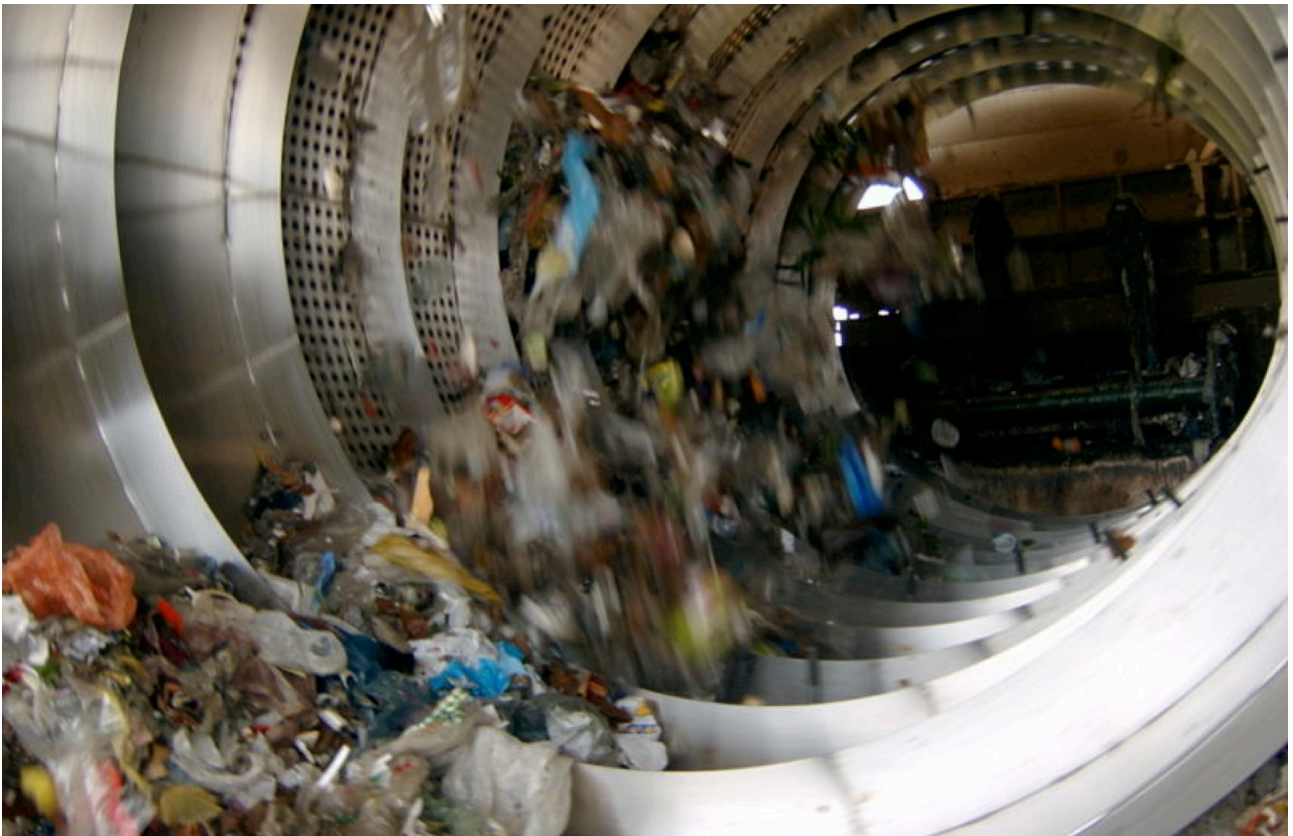
Figure 3. Waste trommel in operation (Photo: courtesy of Spelthorne Borough Council, UK)
