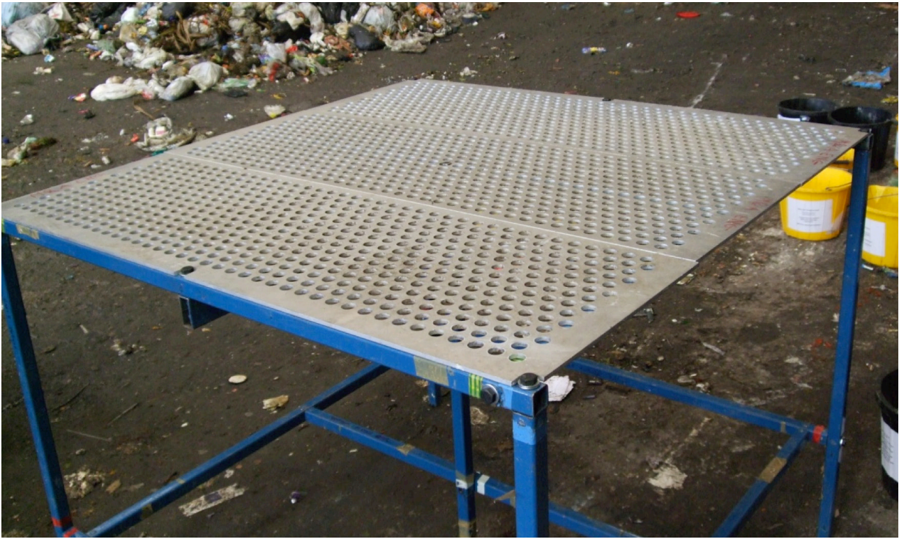
Figure 5. Waste sorting table with a network of 20mm diameter holes
