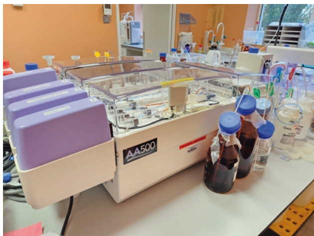
Figure 15. Photo of SEAL Instrument for low-level nutrient analysis
