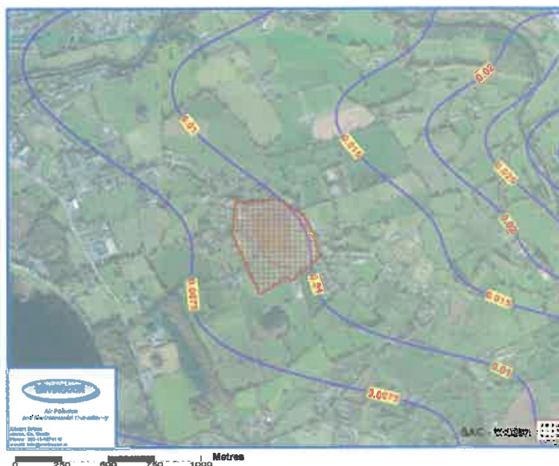
Figure 3: Predicted annual N deposition rates in the locality of Sheheree Bog due to emissions from the asphalt plant. (kgN/ha/yr)
