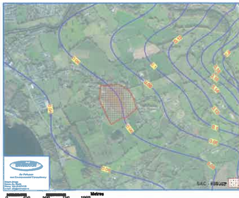
Figure 2: Predicted annual average SO 2 concentrations in the locality of Sheheree Bog due to maximum emissions from the asphalt plant. ( \mu\text{g}/\text{m}^3 )
