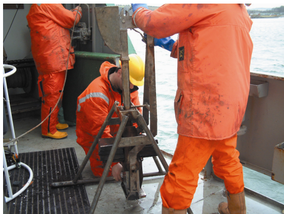
Sediment sampling using a Reineck box corer
