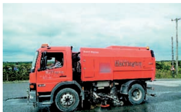
Figure 3.6. Vacuum road sweeper (Frank Harrington Ltd, Carrowscoltia, Co. Mayo).
