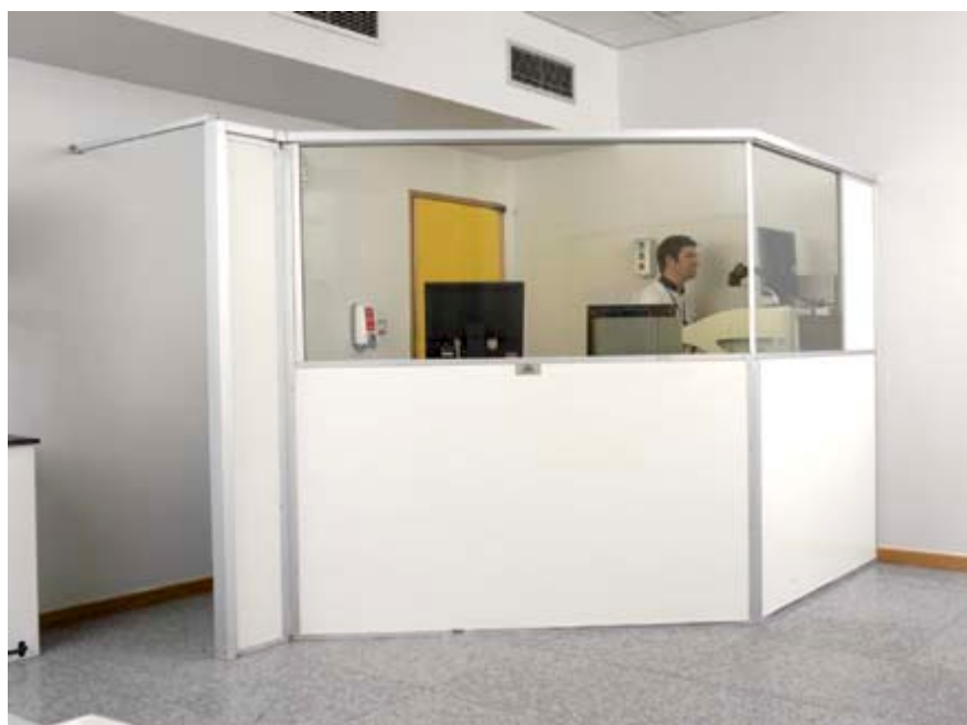
Photo 3.1: Fixed operator's screen
