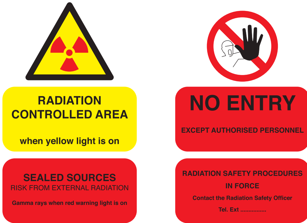
Figure F. 3: Sample radiation warning sign for area containing sealed sources (private communication, Cork University Hospital, 2008)
