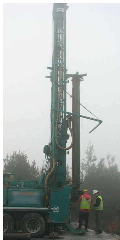
Figure 6.4 Drilling in a Poorly Productive Granite Aquifer, Co. Galway
