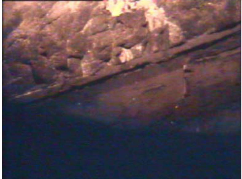
Video camera view of shale and limestone contact
