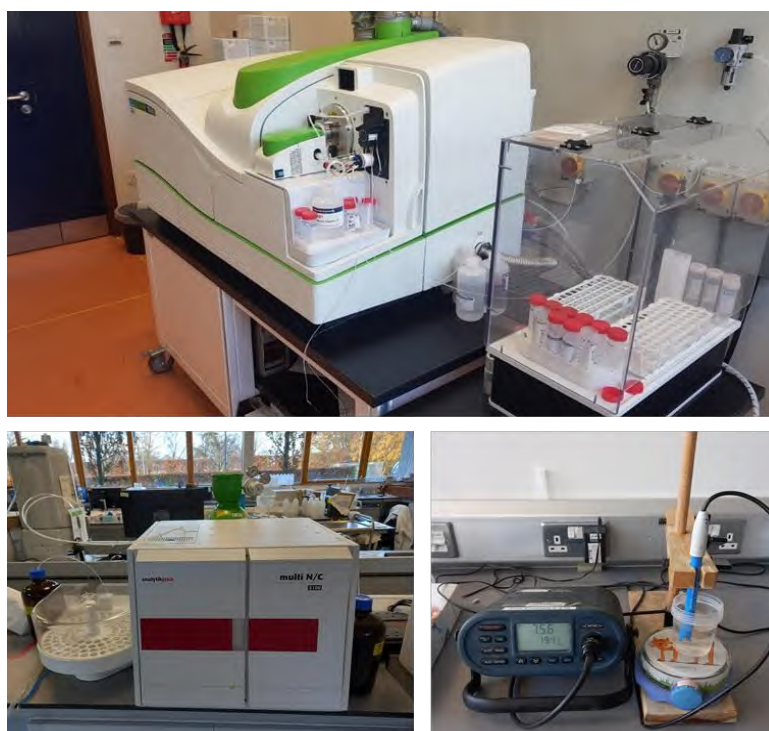
Figure 7 Perkin Elmer 350x ICP-MS instrument (metals analysis), Analytik Jena multi-N/C 3100 (DOC analysis), Multimeter WTW 197i (pH analysis).
