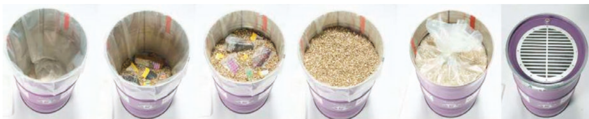
Figure 15: Sample procedure – filling a lined drum with waste Li-ion batteries and vermiculite packing
