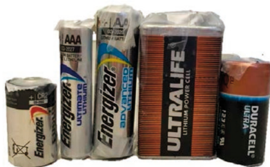
Figure 12: Waste lithium batteries with taped terminals 17
