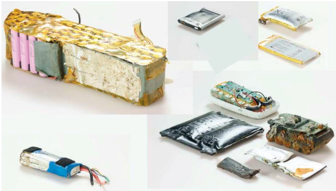
Figure 13: Examples of damaged batteries 21
