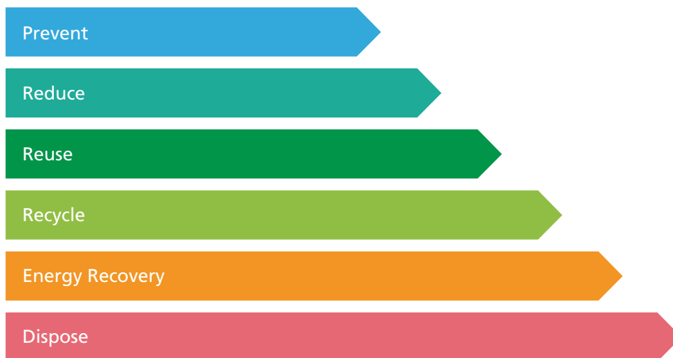
Figure 3: The waste hierarchy, showing the order of preference for actions to reduce and manage waste. Source: EPA.
