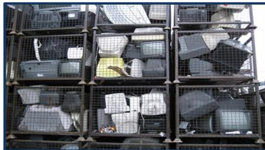
Figure 2. WEEE in cages awaiting treatment
