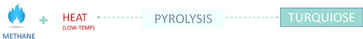
Figure 2.12. Simplified process of turquoise hydrogen production.
