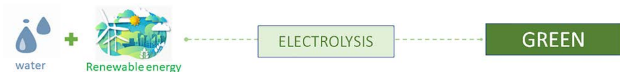
Figure 2.9. Simplified process of green hydrogen production.
