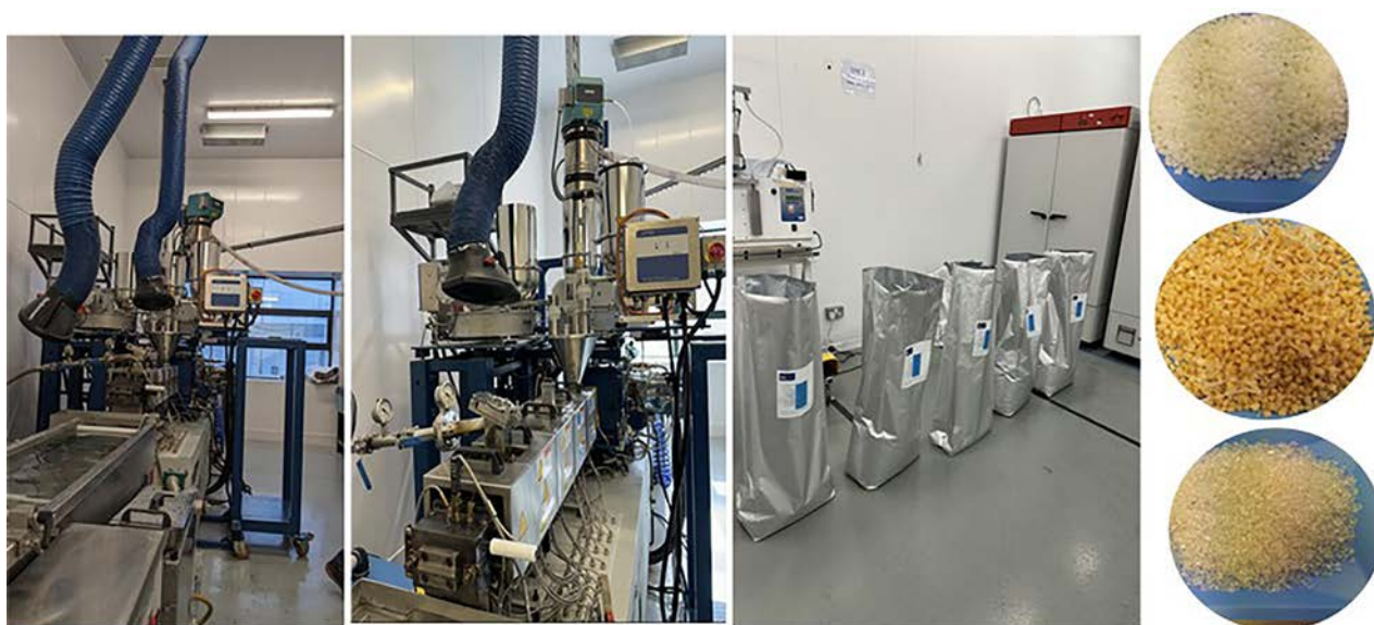
Figure 3.3. Scaling up utilising twin-screw extruders for biocomposites at IPC.
