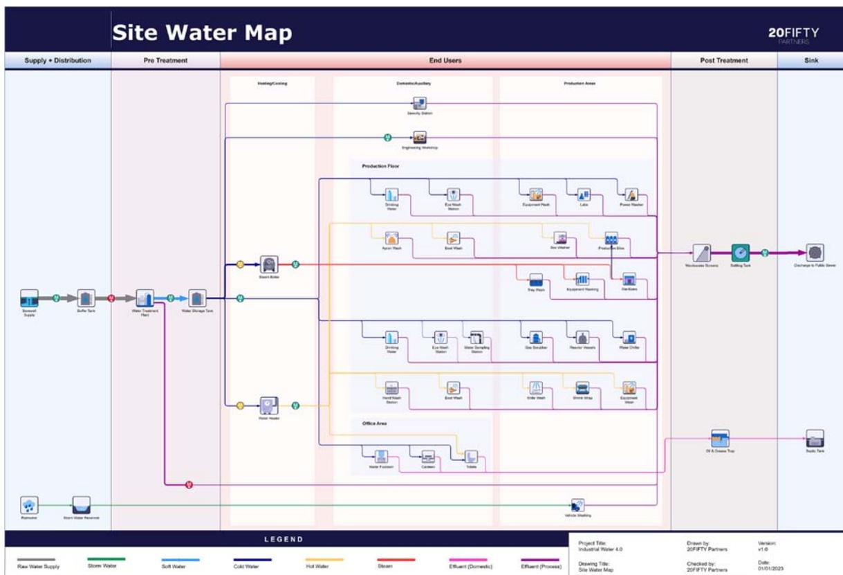
Figure 3.4. Example of a detailed site water map.
