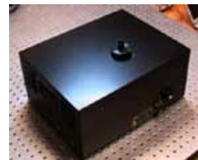
Figure 2.5. Waveband Integrated Bioaerosol Sensor model number 4 (WIBS-4).
