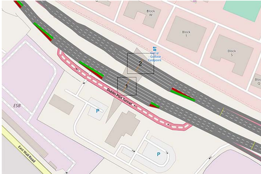
Figure 6.6. Created node features in the VISSIM model: (1) indicates the NB toll and (2) shows the SB toll.
