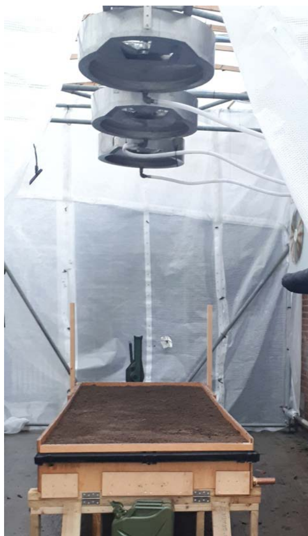
Figure 3.5. Experimental rig for overland flow tests.
