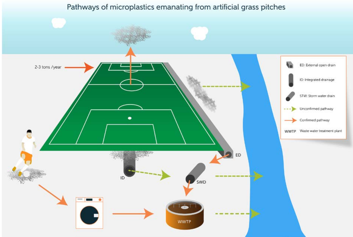
Figure 2.5. A conceptual diagram of inflow and outflow of rubber crumb from AstroTurf pitches.
