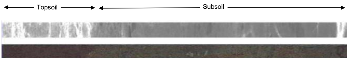
Figure 3.4. Optical image and X-ray of a soil core to a depth of 1 m.
