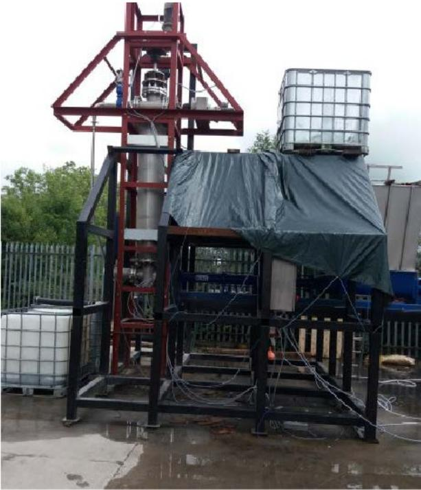
**Figure 3.11. High-pressure pilot filtration rig.**
