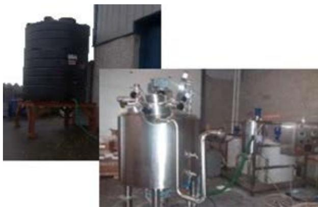
Figure 3.16. Pilot-scale struvite unit.
