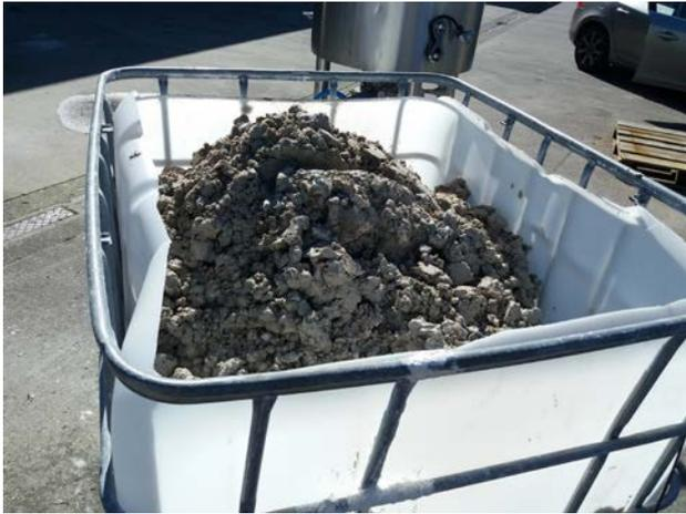
**Figure 3.2. Struvite collected from County Limerick landfill tests.**
