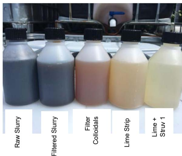
**Figure 3.19. Slurry liquor samples progressively clarified by screening followed by filtration, liming and struvite precipitation.**
