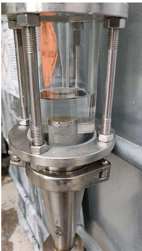
**Figure 2.3. Sparging ammonia vapour through water column.**
