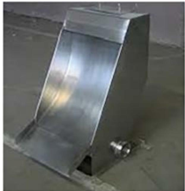
Figure 3.5. Vibrating gravity screen for bulk solids dewatering.
