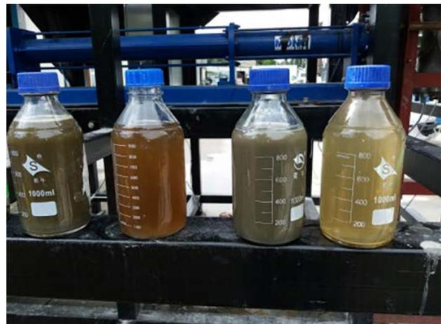
**Figure 3.12. Filtration results using different blends of filter aid. The two bottles on the left show the results achieved using only a coarse filter aid and those on the right show the results achieved with the addition of the fine filter aid. The first and third bottles from the left contain the unfiltered process medium (including filter aid) and the second and fourth contain the filtrate.**
