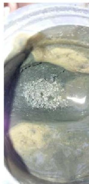
**Figure 3.10. Colloidal solids on filter bed.**
