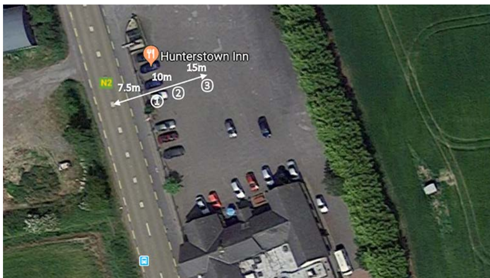
Figure 4.5. Experimental set-up for validation outside an agglomeration. Note: this Google image is used for illustrative purposes only and does not reflect in situ field conditions. No vehicles were present in the vicinity of equipment during the direct measurement period. Maps data: Google © 2019.
