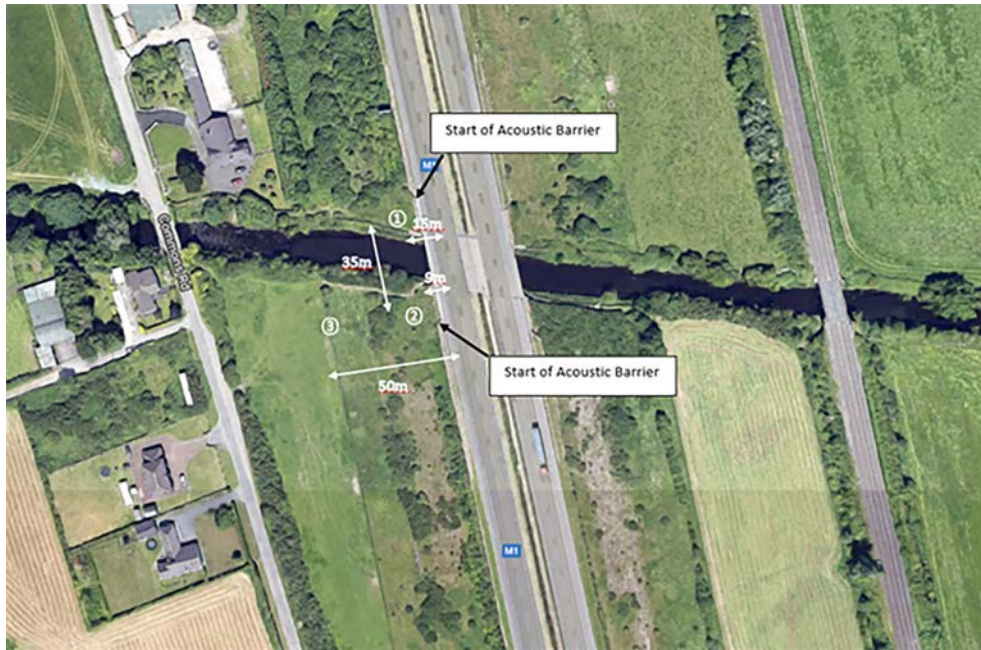
Figure 4.4. Experimental set-up for validation outside an agglomeration. Maps data: Google © 2019.
