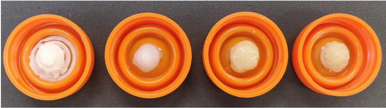
Figure 4.7. The four resin composite dental filling materials after light polymerisation, from left to right: Ceram.X, manufactured by Dentsply Sirona; SDRflow+, manufactured by Dentsply Sirona; Filtek, manufactured by 3M; and Herculite XRV, manufactured by Kerr Dental.
