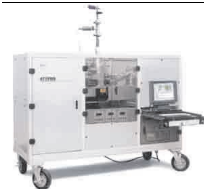
Figure 2.5. The Aerosol Time-of-Flight Mass Spectrometer (TSI 3800) used in the experimental work at University College Cork.
