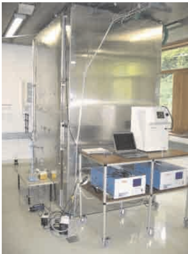
Figure 2.1. The 6,500-l atmospheric simulation chamber at University College Cork.
